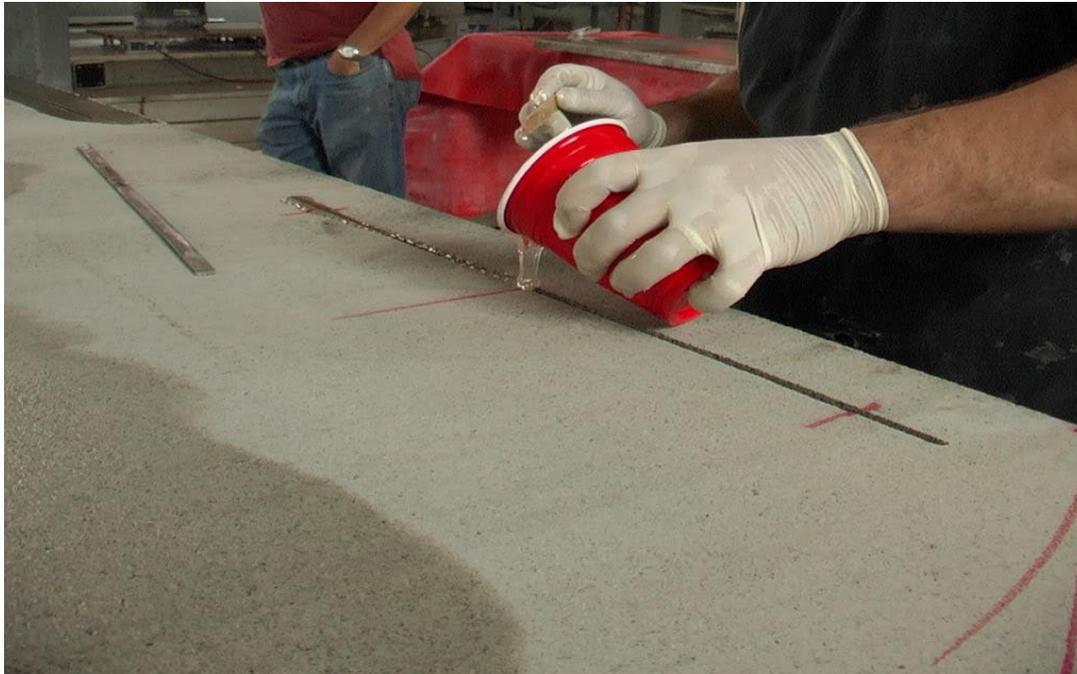
We cut a slot for a steel rod or flat bar to sit in..
